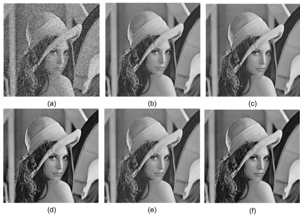
Fig. 2. LENA image (a) corrupted with 20% salt-and-pepper noise, restored images using, (b) SMF, (c) PSMF (d) DBA, (e) NIDF, and (f) Proposed
