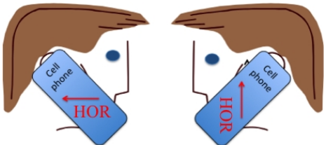
Fig. 1. Illustration of the fact, that the vertical direction relative to handheld phone-type terminal is undefined. A horizontal arrow and the text “HOR” is taped on to the phone when this is held on the right side of the head (left drawing). We see that this taped arrow and “HOR” text becomes vertical when the phone is held on the left side of the head (right drawing).
