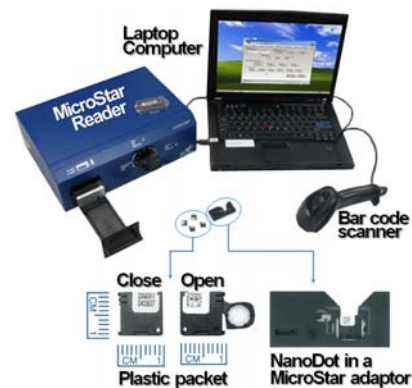
Fig. 1. InLightTM optically stimulated luminescence dosimeters (OSLDs) system.
