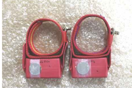
FIGURE 2. GCT wildlife tracking system(225g ; GCT-M1, Korea institute of environmental ecology, Daejeon, Korea)
