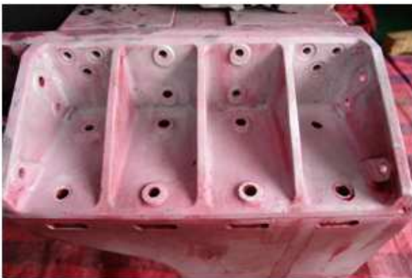
Fig. 10 Crack inspection of casting block and magnet pole bracket connection
