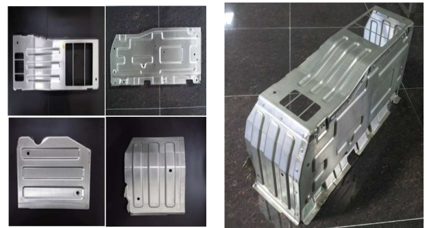
Fig. 7(a) Parts of battery pack case Fig. 7(b) Assembly of battery pack case
