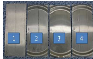
Fig. 11(a) Test specimen before the salt spray test; (1) before forming, (2) 230°C(hot-forming, HF), (3) 250°C(HF), (4) 270°C(HF)
