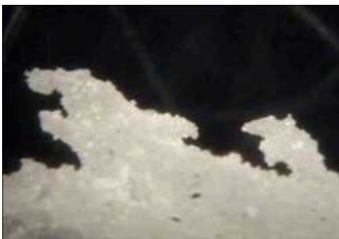
Fig. 8. Optical microscopy image of the ridge on the surface of SBS/HSR (80/20) blend.
