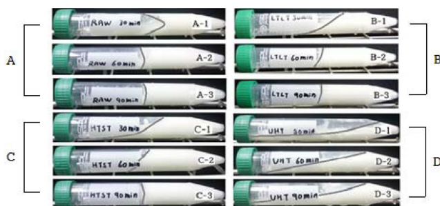
Fig. 1. Results of the rennet coagulation test on raw milk and some commercial milk products after incubation for 30(1), 60(2), and 90(3) min, respectively. A1-A3: Raw milk, B1-B3: LTLT (Low temperature long time) treated milk, C1-C3: HTST (Hight temperature short time) treated milk, D1-D3: UHT (Ultra high temperature) treated milk.
