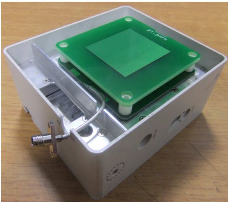
Fig. 11. Photograph of proposed repeater antenna
