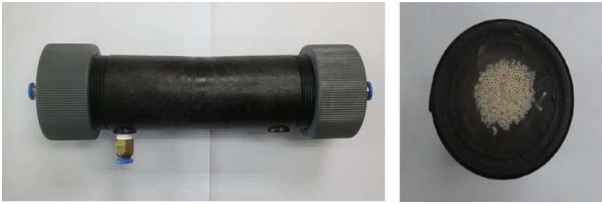
Fig. 2. Photograph of the test module and housing for hollow fiber membrane.
