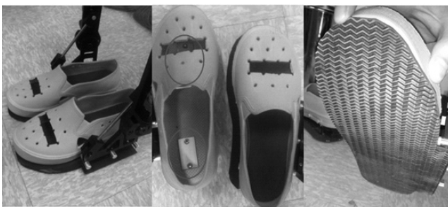
Fig. 12 Pressure sensors and anti-sliding pad
