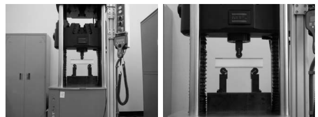
Fig. 2 Experimental setup of bending test
