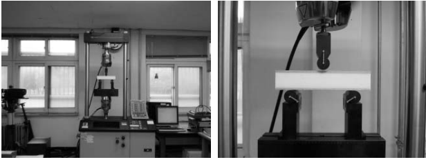
Fig. 3 Experimental setup of Fatigue test
