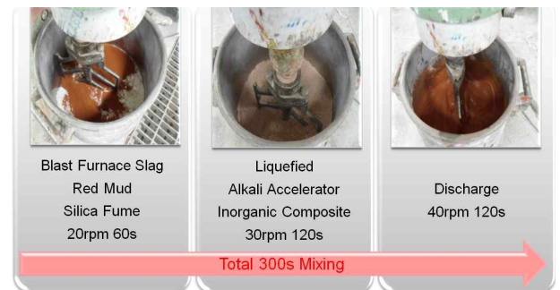
Figure 6. Mixing process of inorganic composite
