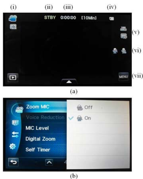
Fig. 4. Snapshot of the graphic user interface (GUI) designed for the proposed video-zoom driven audio-zoom algorithm (a) main GUI configuration, (b) audio-zoom mode GUI configuration.
