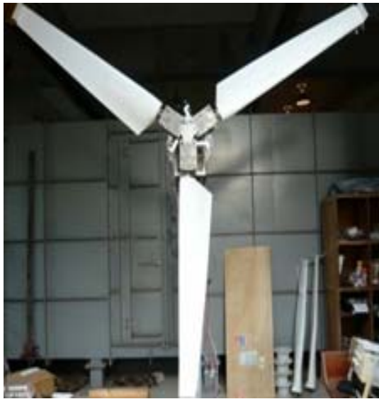
Fig. 3. Small-scale wind turbine system.
