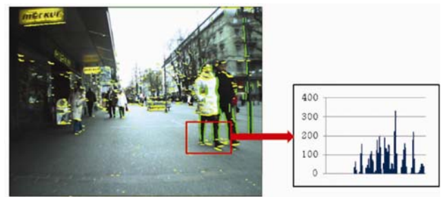
Fig. 4. Example of the symmetry histogram. The vertical symmetry is stronger if the histogram has a higher value.
