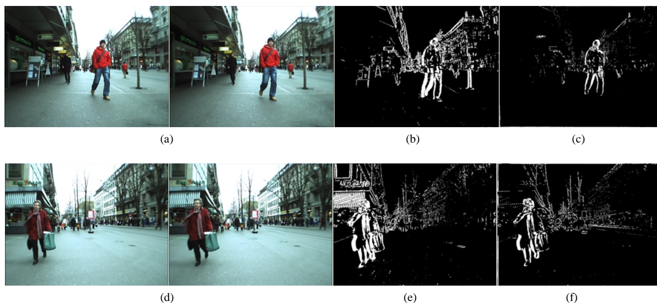
Fig. 2. Comparison of difference images (a), (d) Original images (2 consecutive images); (b), (e) the conventional difference images; and (c), (f) the proposed difference images using GME.
