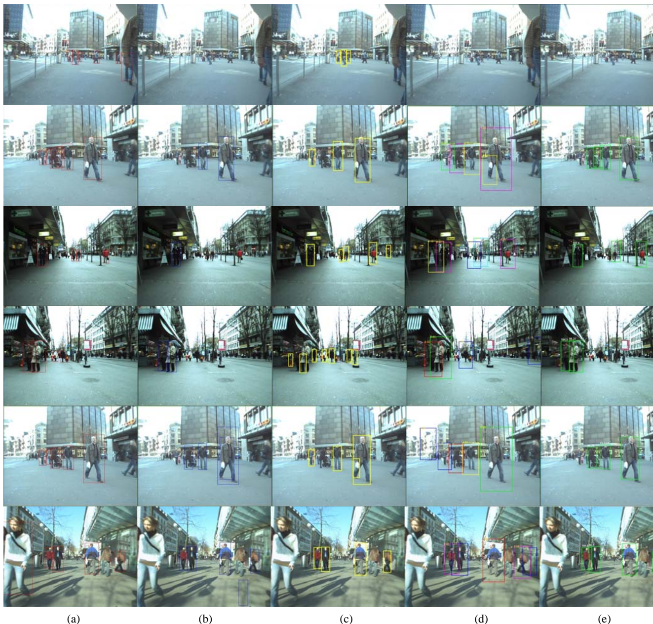
Fig. 8. Comparison of the proposed algorithm with the conventional algorithms (a) proposed algorithm, (b) Felzenszwalb et al. [3], (c) Schwartz et al. [19], (d) Maji et al. [20], (e) Dollar et al. [7].
