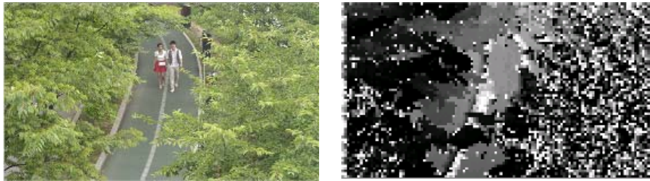
Fig. 9. Snapshot of the stereoscopic video that results in low MOS obtained when the frame boundary areas in the stereoscopic video frames are perceived to be excessively protruded.
