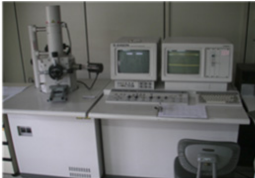
Figure 11. Electron microscope (SEM).
