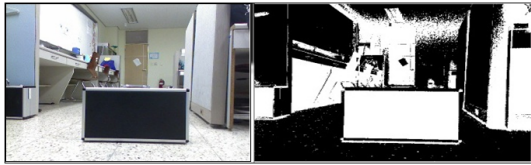
[Fig. 6] Color image binarization
