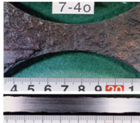
[Fig. 3] Conditions of surface and cross section of rusted specimen[3]
