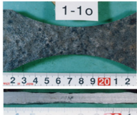
[Fig. 2] Conditions of surface and cross section of rust removed specimen
