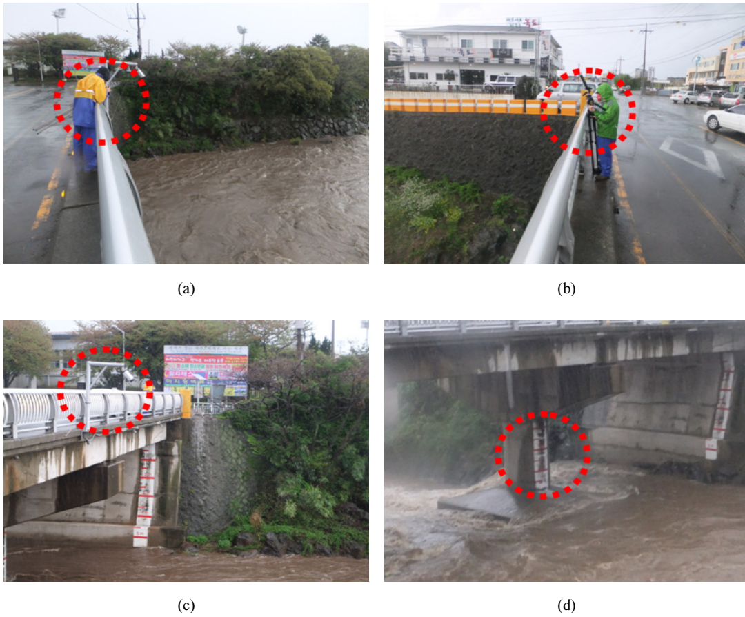
Fig. 5. Various velocity measurement systems in the study site : (a) Surface Image Velocimetry(SIV); (b) Electromagnetic surface current meter; (c) Kalesto; (d) Staff gauge.
