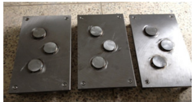
Photo 2 Steel Specimens for Bond Strength
