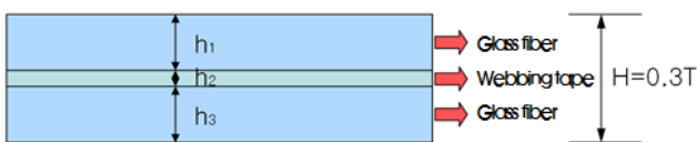
Fig. 11 Inhomogeneous GP Composite fiber faults
