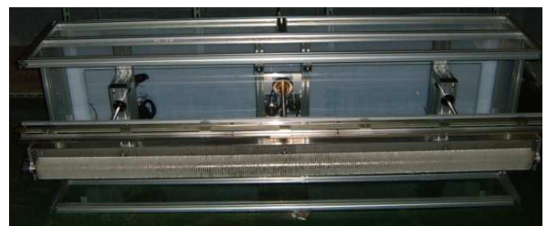
Fig. 3 Prototype of a cleaning tool for moving forward and backward
