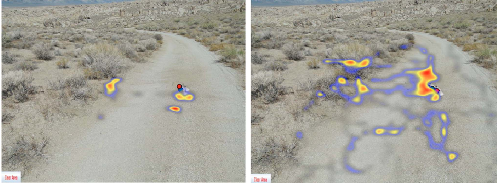
Fig. 7 Gaze density difference between experts (left) and novice (right) in IED detection task. Gaze location of experts is more concentrated on certain locations than that of novices [42]
