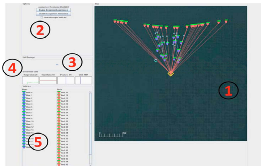
Fig. 6 Interface of RESCHU-SA (Research Environment for Supervisory Control of Heterogeneous Unmanned Vehicles - Swarm Attack): 1-area of operation; 2- assignment mode panel; 3-HVU damage level indicator; 4- physiological data monitor; 5-blue and red health monitoring panel [31]
