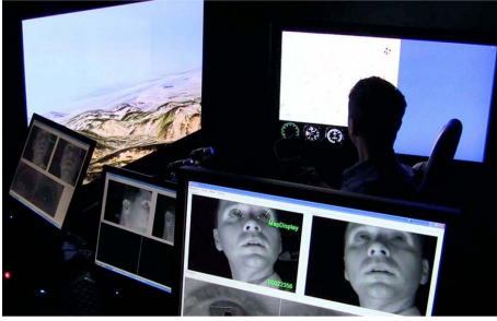
Fig. 1 Overland navigation experimental set-up with two remote eye-tracking systems
