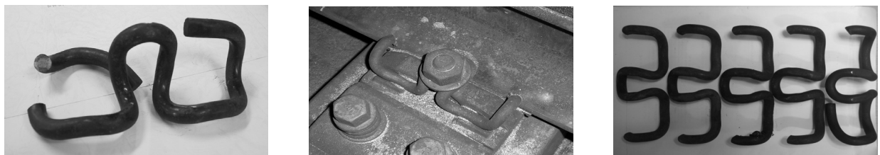
Fig. 4. Photograph of the fractures for in-situ tension clamp
