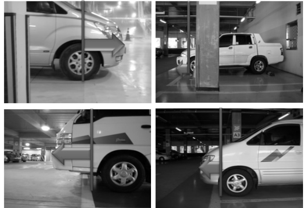
Fig. 7. Examples of Violation of Parking Space Section by Increased Vehicle's Dimension
