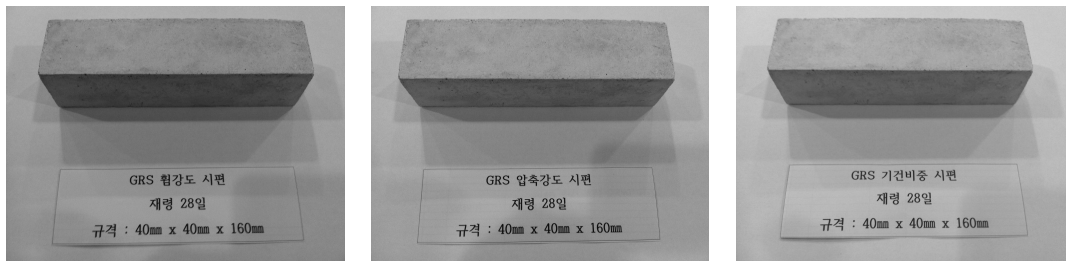
Figure 1. The specimens for GRS performance test.
