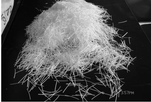
Figure 3. Shape of polypropylene fiber.
