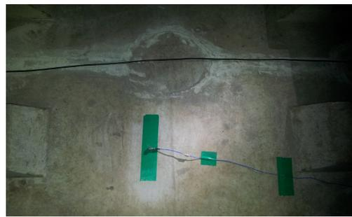
Fig. 4 Survey Acceleration Response of Concrete Bed
