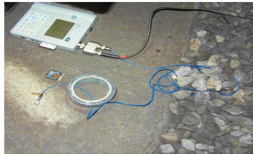
Fig. 5 Survey Acceleration Response of Ballast Bed
