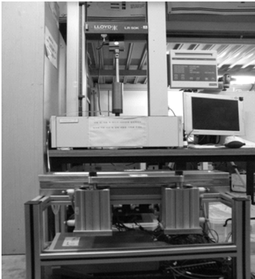
Fig. 1. Fluid injection pump controlled by UTM (universal test machine).
