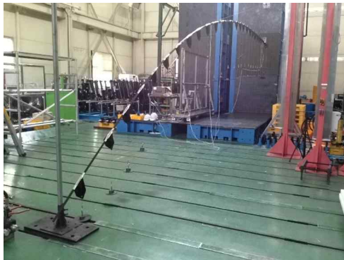
Fig. 18 Static Strength Test - 100% Test Loads
