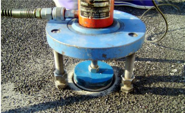
Fig. 12 Testing for Adhesive Strength of Bio-Polymer Concrete
