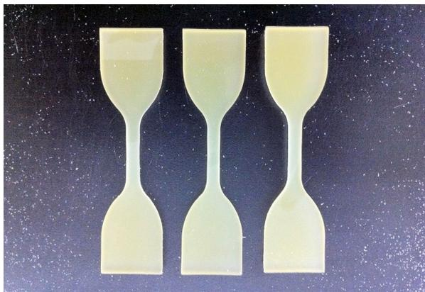
Fig. 2 Cured Bio-Polymer Binder for Tensile Strength Testing
