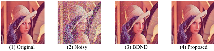
Fig. 7. Outputs for Lena (color) image for noise model 2 (40% impulse noise density {high density=30, low density=10}, m=30 )
