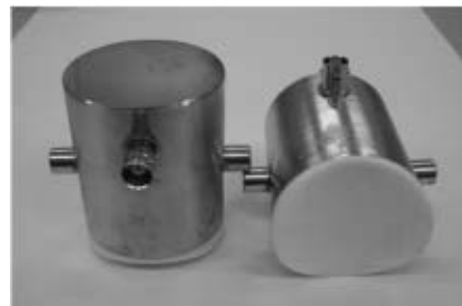
(a) Ultrasonic transducer
