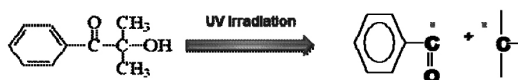
Fig. 2. Cleavage of hydroxydimethyl acetophenone as a photoinitiator in the presence of UV light[27].
