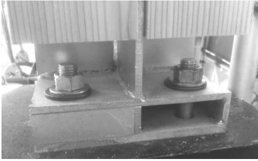
Fig. 11. Direct bolting of the connector upper plate.
