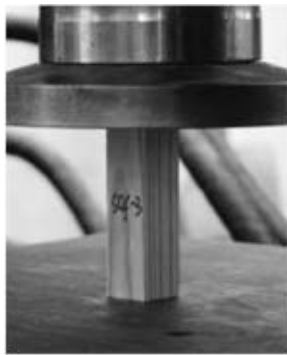
Fig. 3. Photograph of compressive test.
