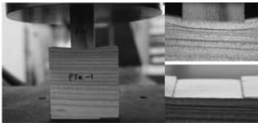
Fig. 4. Photograph of partial compressive test.
