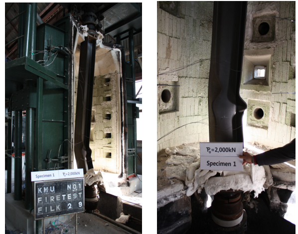
Fig. 3 The failure mode of test model B(S-1)
