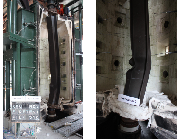
Fig. 2 The failure mode of test model A(S-2)
