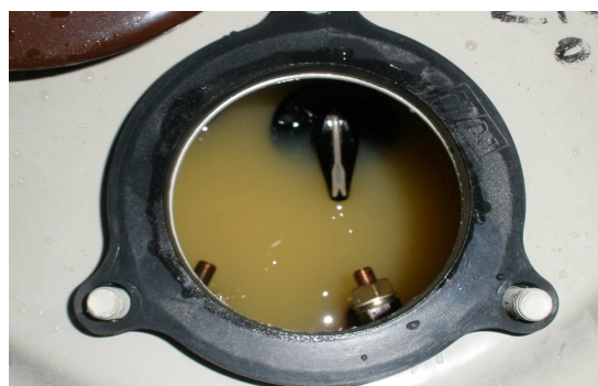
Fig. 1. The solidified status of the natural ester fluid
