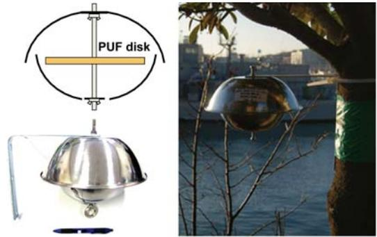
Fig. 1. Passive air sampler (PAS) equipped with a polyurethane foam (PUF) disk.
