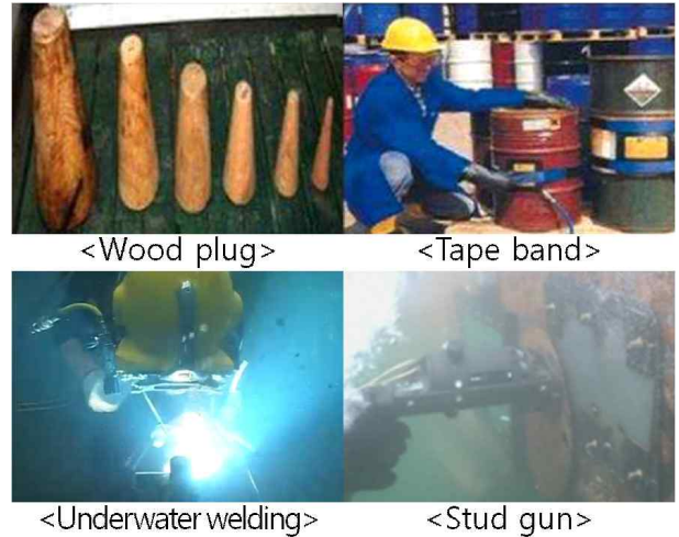
Fig. 1 Existing equipments for liquid spill stopping
