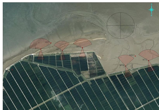
Fig. 4. Installation Positions of Wind Turbines.
