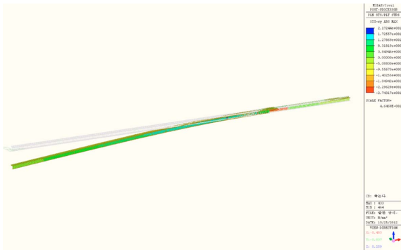
Fig. 12. Shear stress of stool member.
