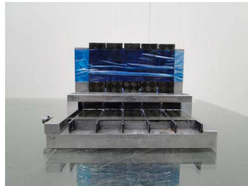
Fig. 3. Bonding assembly tool for L-type specimen.
