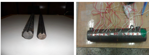
Fig. 8 Grooved rebar and strain gage attachment on sleeve
