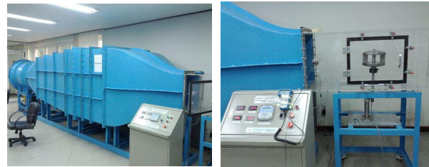
Fig. 6 Prototype model installed in the wind tunnel
