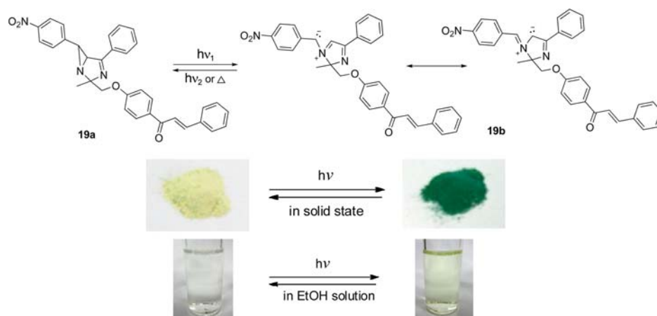
Scheme 2. Photochromic reaction in the solution and solid states.
