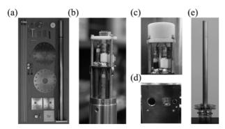
**Figure 1.** The 800 MHz NB lab-built strip-shield low- $\epsilon$  solid-state NMR probe. (a) Parts of the probe assembly. (b) The completed probe head, the strip shield was used to prevent heating of the bicelle sample and the coil. (c) PTFE coil cap for the sample. (d) Probe heat sensor and heater for temperature control. (e) The whole probe.
