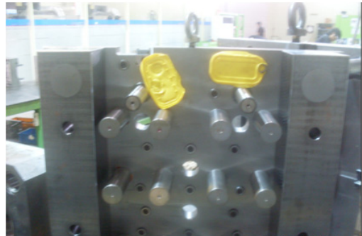
Fig. 4. defect product entry (Pushing pin worn on the phenomenon)
