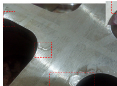
Fig. 3. Core components occurs in the appearance of wrinkles
